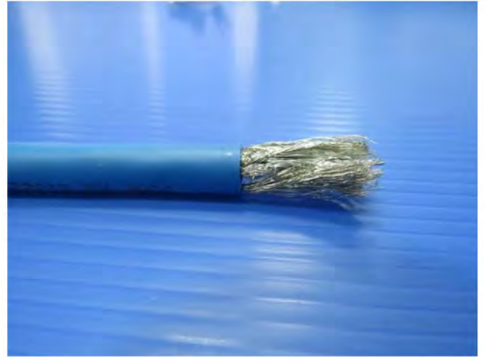
2. Strip 20mm sheath from the cable
